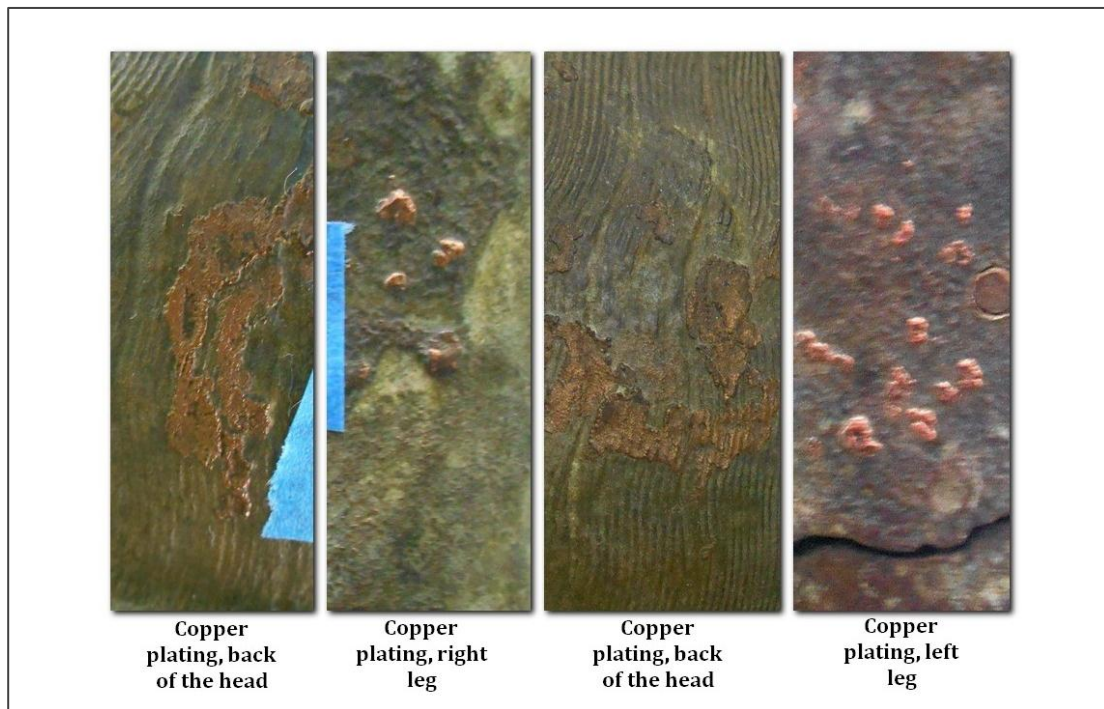
Figure 8. Example of copper platings throughout the surface of the statue
