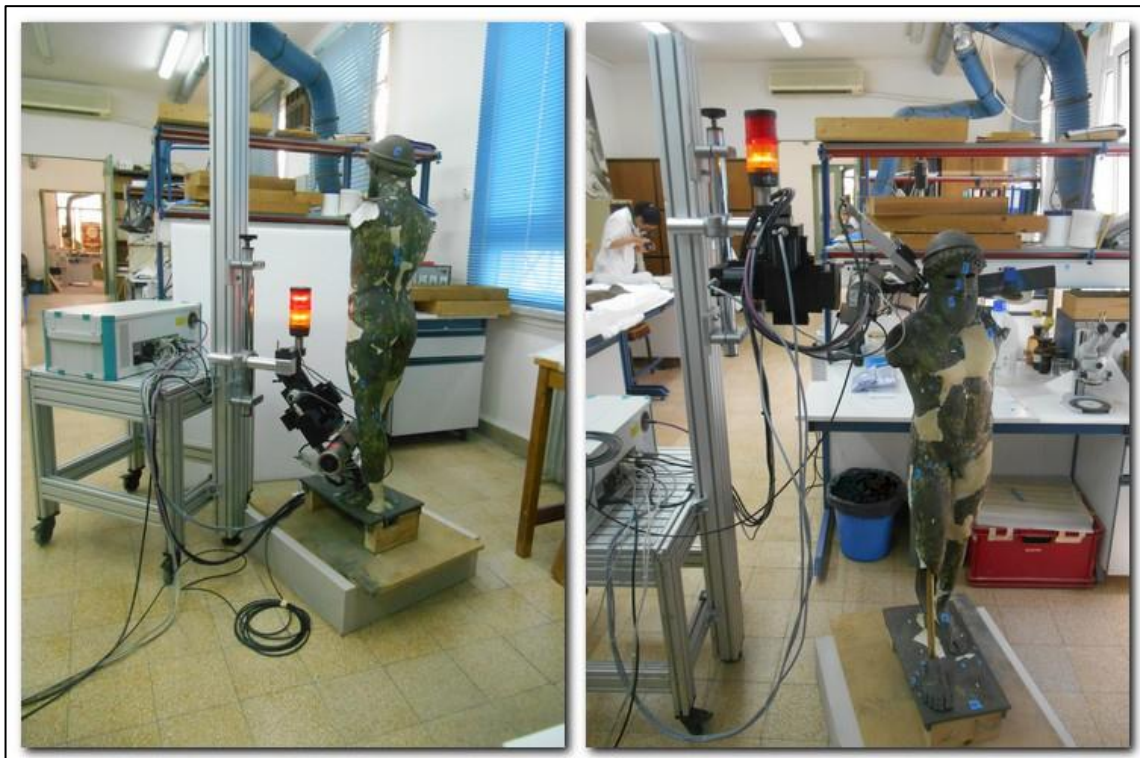
Figure 10. The configuration of the apparatus during the analysis of the nape and left foot. As it can be seen in the photo, the head of the spectrometer changed angle so as to better reach the surface to be analyzed.
