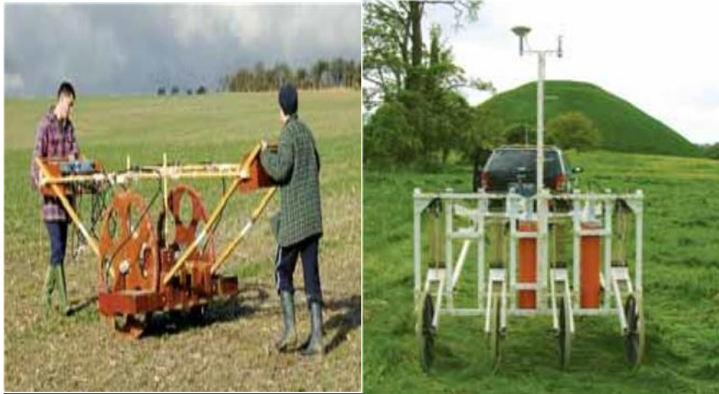
Fig.8 (left)Cart mounted magnetometer systems: four caesium sensors mounted at 0.5m intervals(Jones 2008)
