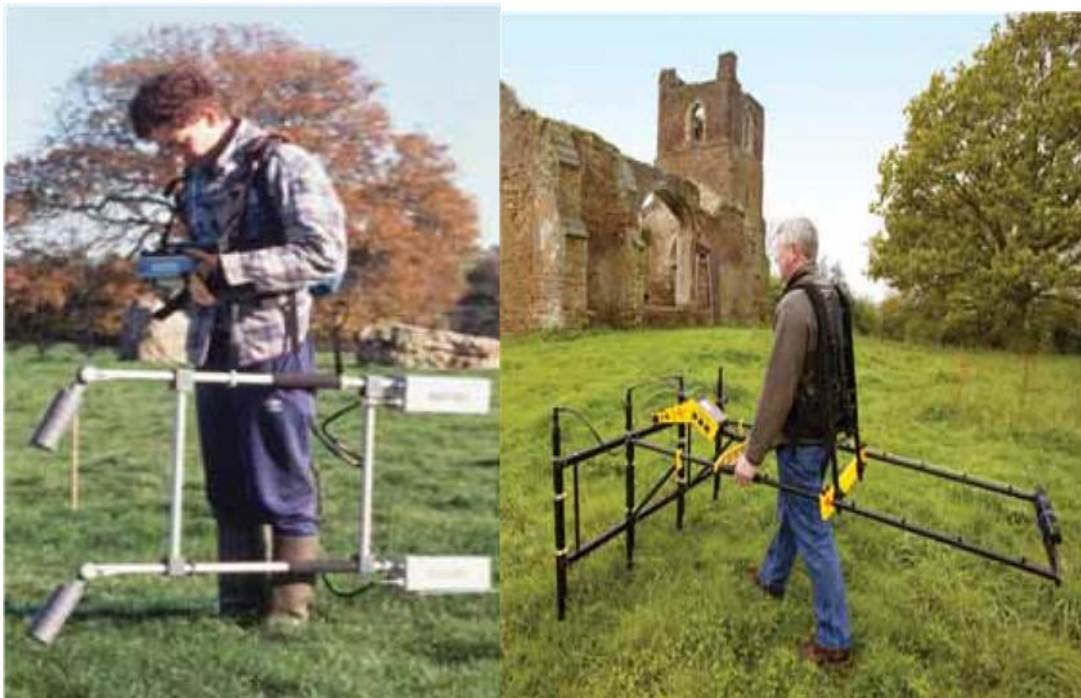
Fig.6Acaesium magnetometer (Jones 2008)
