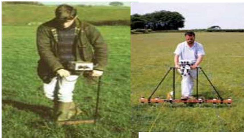
Fig.13/14 Geoscan RM15 earth resistance meter in use (left) in standard twin electrode configuration; (right) with a multi-electrode array addressed via an MPX15 multiplexer (Jones 2008)
