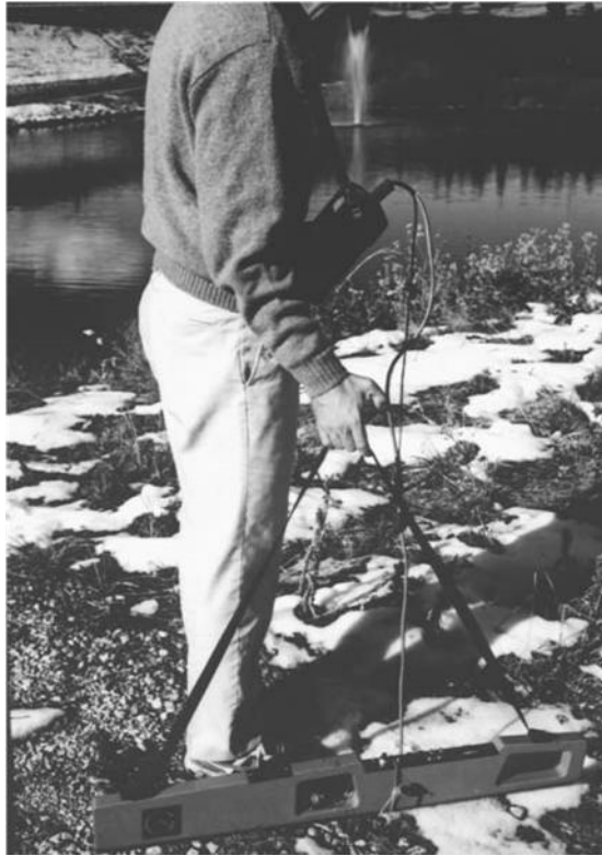
Fig.15 Electromagnetic (EM) instrument with one meter separation between the transmitting and receiving coils (Davenport 2001).
