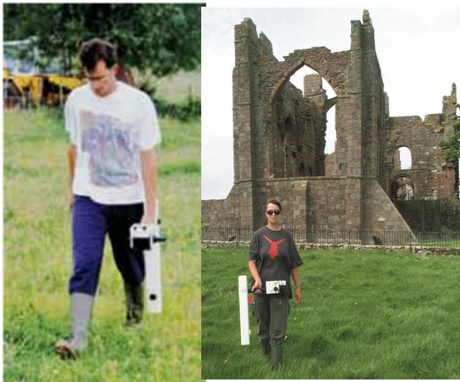
Fig.2/ 3. Handheld signal fluxgate magnetometers (Jones 2008); (Gaffney 2002).
