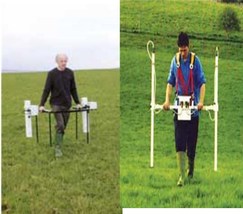
Fig.4(left)Handheld magnetometer in dual sensor configuration (Jones 2008)
