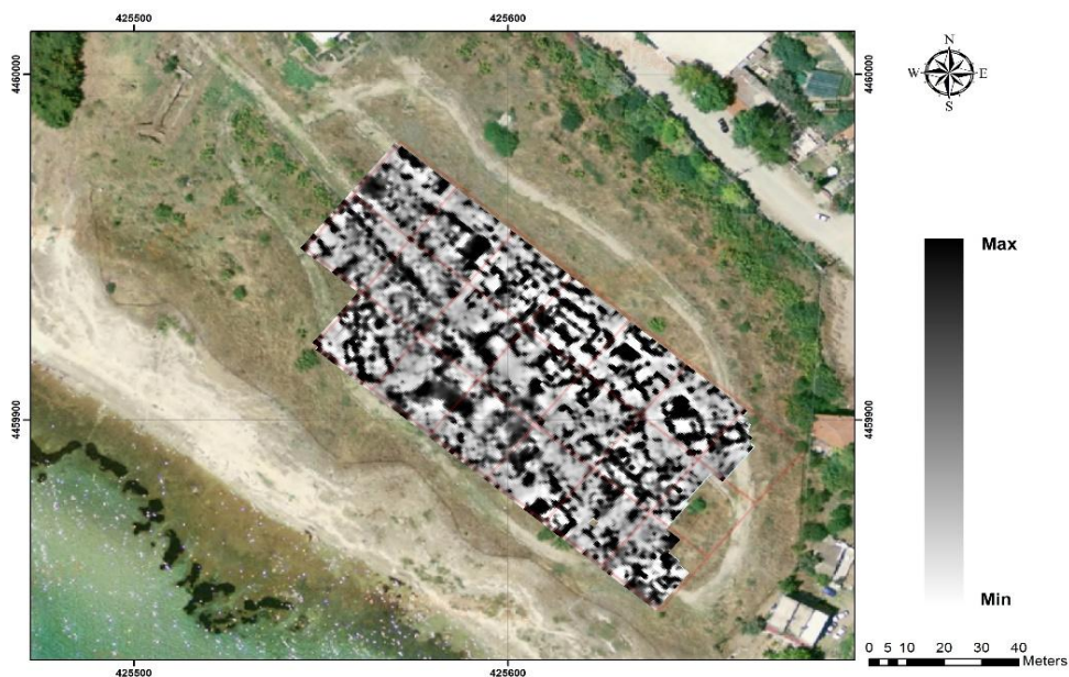
Fig.31 The urban planning of the Toumba, revealed by the electrical resistivity survey.
