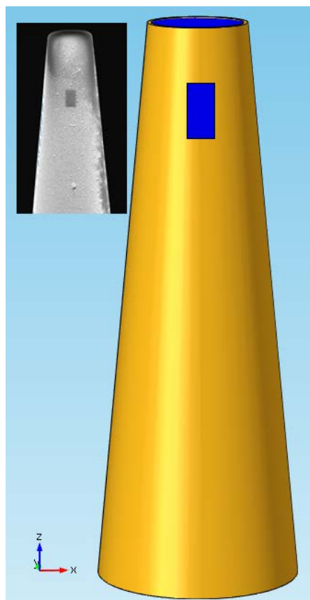
Figure 2-1. A schematic illustration of a gold-coated optical fiber tip with a rectangular plasmonic slot nano-resonator (PSNR) (inset picture: SEM image of a gold-coated fiber tip with a rectangular PSNR).
