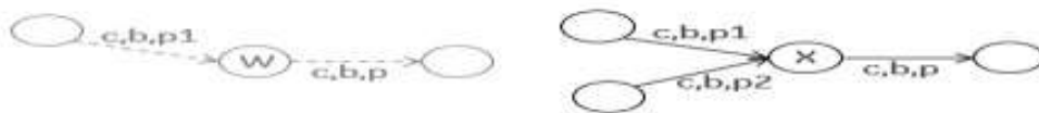
Figure 20 System W fails validation because p1 is onlt subset of p . System X passes validation.
