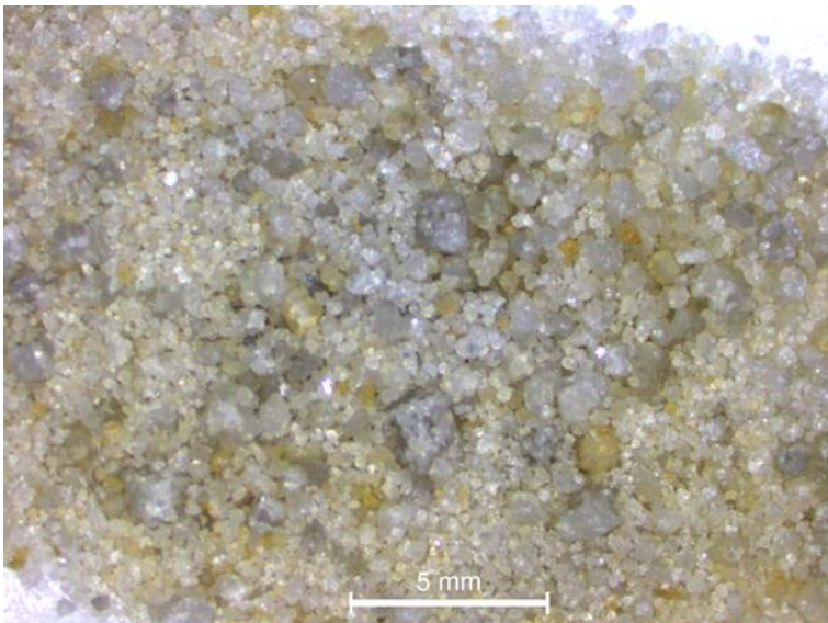
Fig. 10: General photo of the sample. Different sizes of aggregates, mainly of rounded shapes, containing a different number of grains of white, grey, yellowish color.
