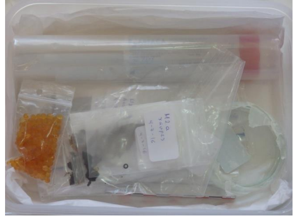
Fig.8: Stored samples in plastic polypropylene box, with antacid paper and silica gel.
