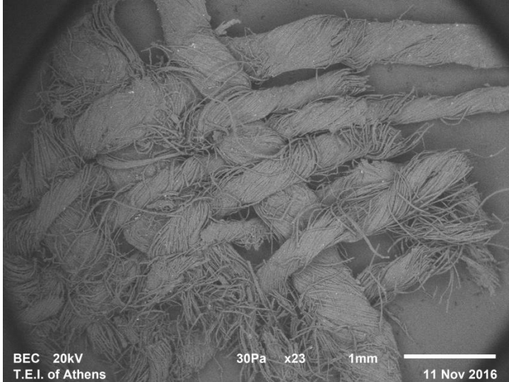
SEM image M2e: Detail of the weaving. Simple weaving, damaged threads and fibers.
