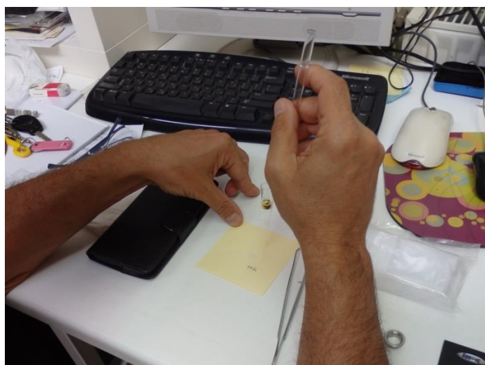
Fig.17: The solution was extracted by the use of glass pipette on the KBr pellet.
