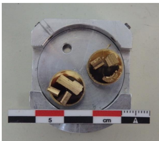
Fig.14: M1i sample were coated with gold for SEM analysis.
