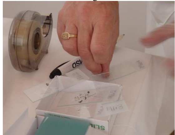
Fig.9-10: Dry swabs (left image) and clear masking tape (right image) for biodeterioration examination.
