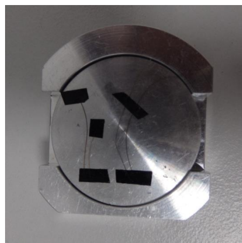
Fig.15: M1h sample. Two hairs were selected for SEM analysis.
