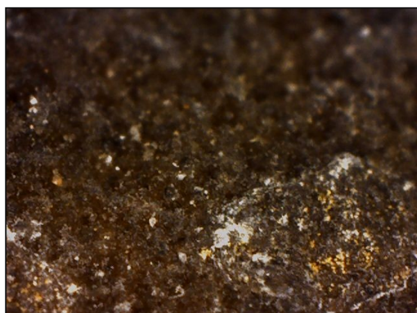
Fig. 27: Black crust on sample B3 (magnification 200×).
