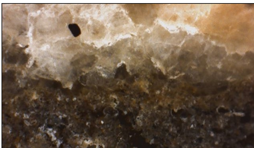
Fig. 24: Interface between the substrate and the innermost dark layer in sample B1 (magnification 200×).
