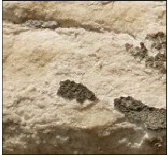
Fig. 10: Thin dendritic black crust on exposed surface after material loss (Ephorate of Antiquities of Athens).
