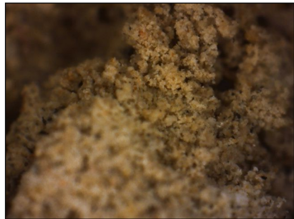
Fig. 20: Detail of intermediate layer in the black crust of sample B1 (magnification 200×).
