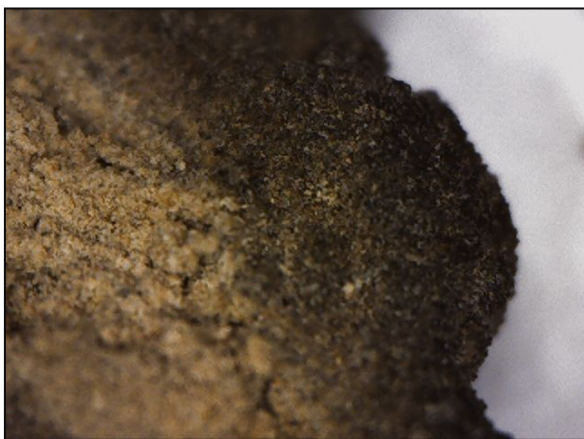
Fig. 19: Gradual change in color and texture of crust on sample B1 (magnification 50×, polarized light).
