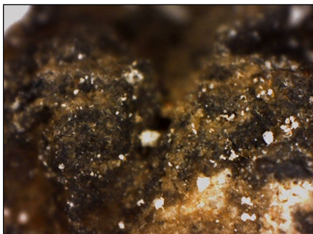
Fig. 35: Dendritic black crust on the surface of sample B5 (magnification 200×).
