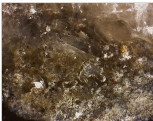
Fig. 33: Interface between the substrate and the innermost crust layer in sample B4 (magnification 200×).
