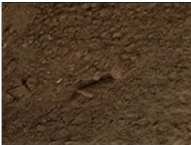
Fig. 8: Contour scaling in context with black crust (Ephorate of Antiquities of Athens).
