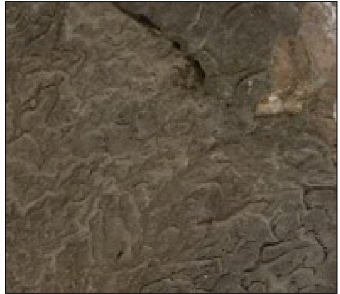
Fig. 12: Thick compact black crust in sampling spot of sample B3 (Ephorate of Antiquities of Athens).
