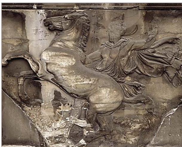
Figure 3 Deposition of aerosols particles on recrystallized calcium carbonate (marble) (YSMA, 2011)
