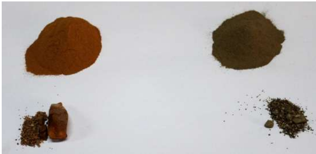
Figure 5. Imaging of the two clay fabrics after the purification with the sieve (top), the unrefined clay soils (bottom)
