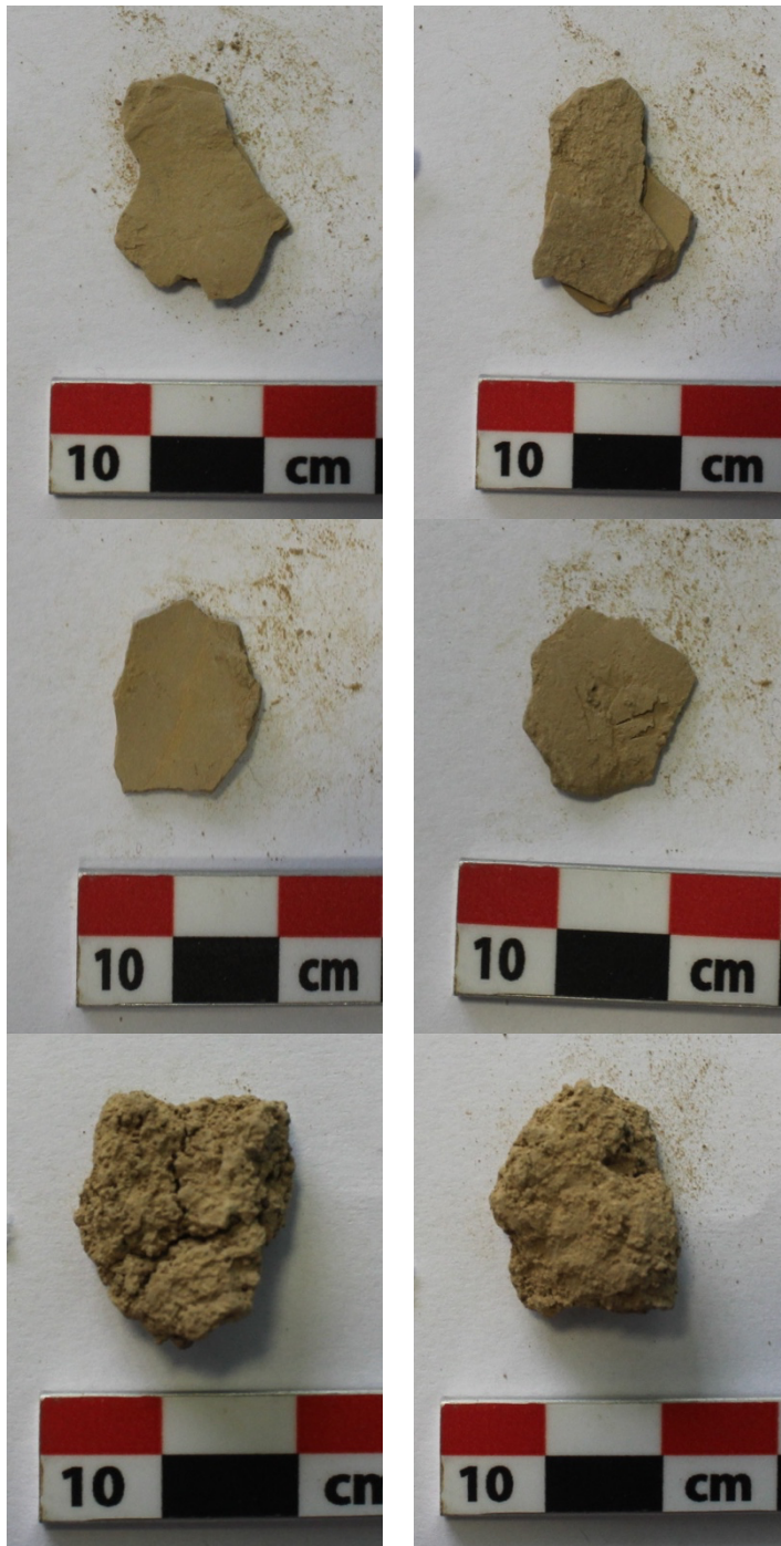
Figure 31: Sample Side Comparison. Comparison of the smooth (left) and rough (right) sides of the Refined Analysis group. (From top to bottom: A1, B1, B4, B6, B7, & C3 5 ).
