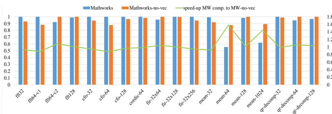
Figure 234: Performance of MathWorks fixed point generated code compared to MathWorks non-vectorized code compiling with Clang on desktop with i7-3820
