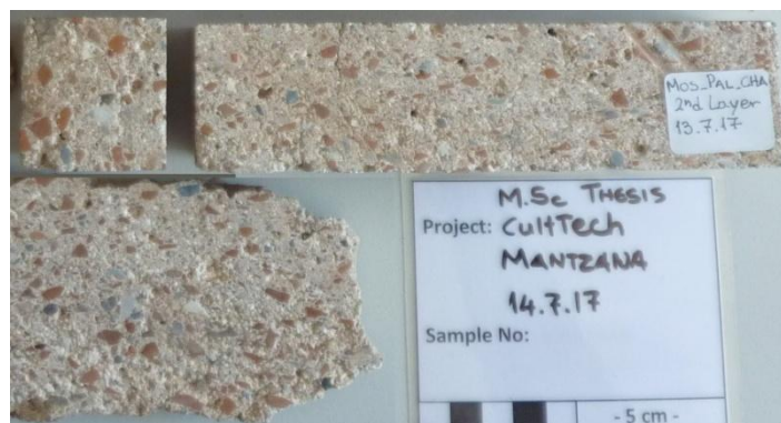
Figure 36. Authentic mosaic mortar rectangular prisms and samples, before mechanical properties tests. (Manzana E.)
