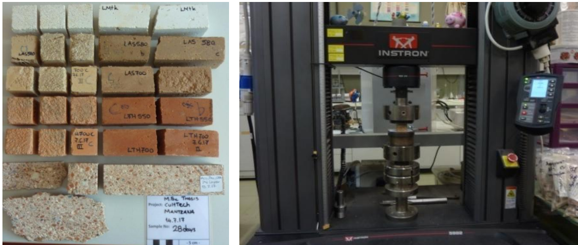
Figure 46. Left: The laboratory lime mortar specimens with ceramic admixtures (Thrapanso & Agios Syllas) and ancient mosaic mortar sample, after the completion of mechanical properties tests. Right: The INSTRON machine of “NCSR DEMOKRITOS” during compressive strength test.
