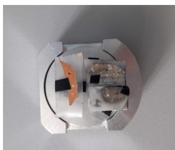
Fig. 15 Samples Carbon Taped and Mounted on the Specimen Holder
