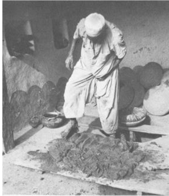
Fig. 2 Mixing and homogenization of clay paste ( Velde & Druc 1999, 19)
