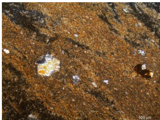
Fig. 24 Representative Microphotograph of thin section sample 2 with Crossed Polars x50.
