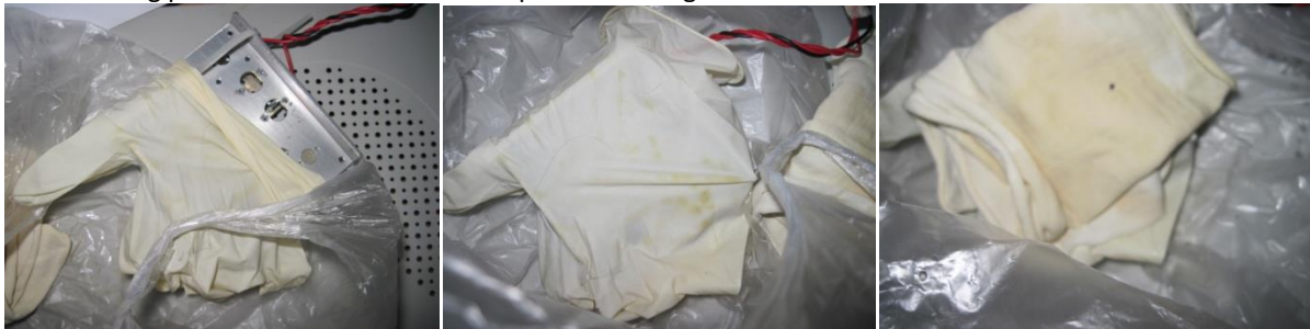
Figure 85. Left to Right: Heated plate partially inside glove, glove after experiment, cloth after experiment
