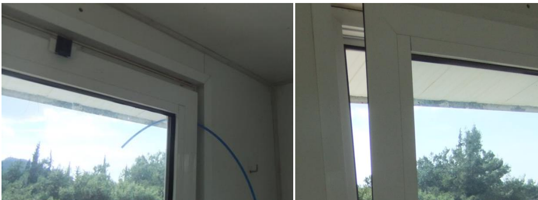
Figure 76. Left: sampling fresh air. Right: different ventilation parameter via different window opening
