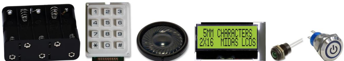
Figure 204: From left to right, battery holder, keypad, speaker, LCD screen, LED indicator, ON/OFF push button.
