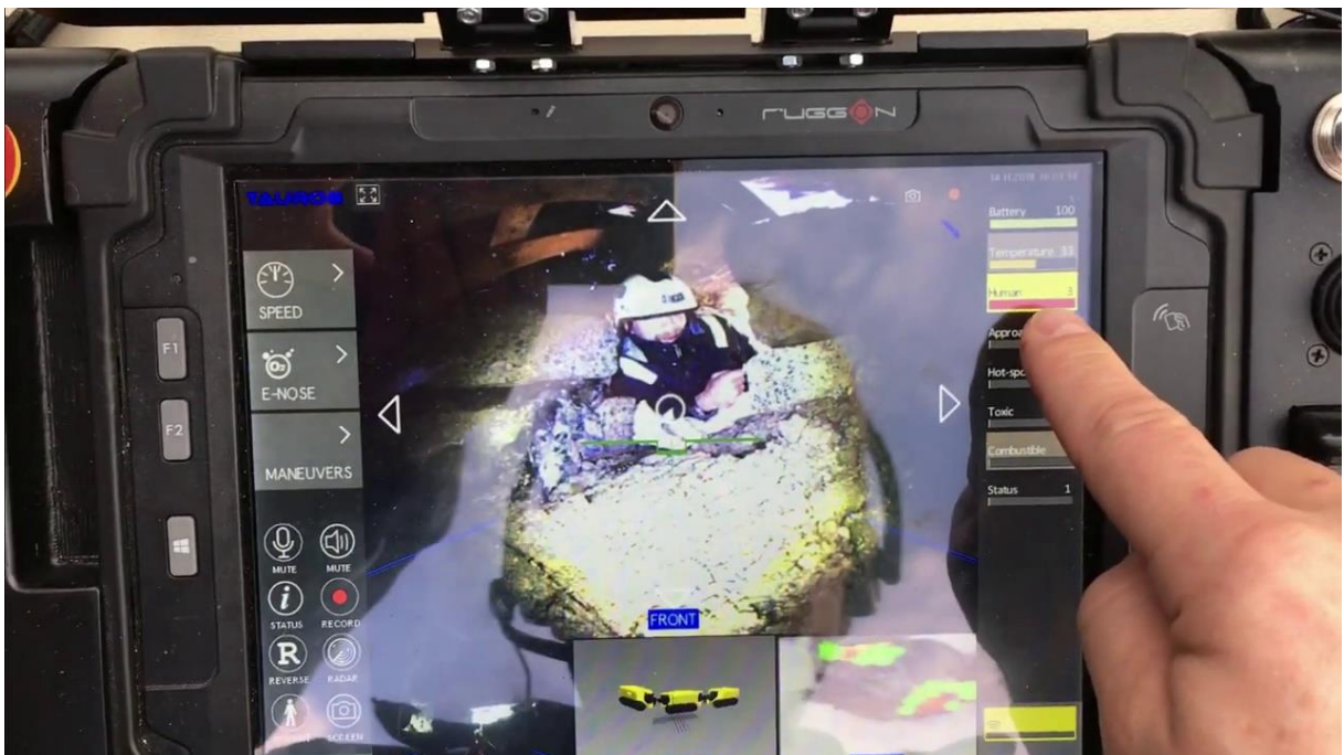
Figure 194. The robotic platform's control interface. On the right is the output of the e-nose, from top to bottom: Human indicator (red = strong indicator, person detected), Approaching indicator, Hot-spot indicator, Toxic indicator, Combustible indicator, Status indicator.
