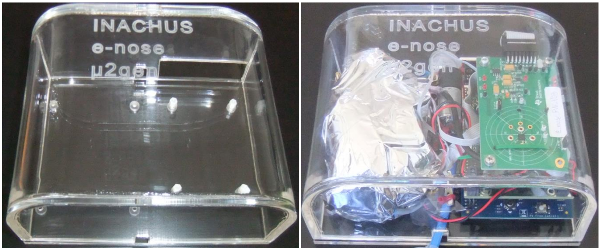
Figure 44. The Plexiglas enclosure (left) and the complete 2 nd e-nose prototype.
