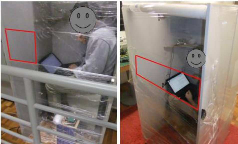
Figure 51. Testing different locations of the e-nose and a larger ventilation opening size 20x60cm
