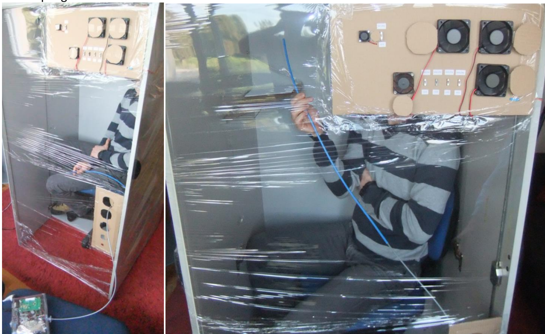
Figure 62. Left: All fans OFF ventilation openings open. Right: All fans ON ~ 1750 LPM.
