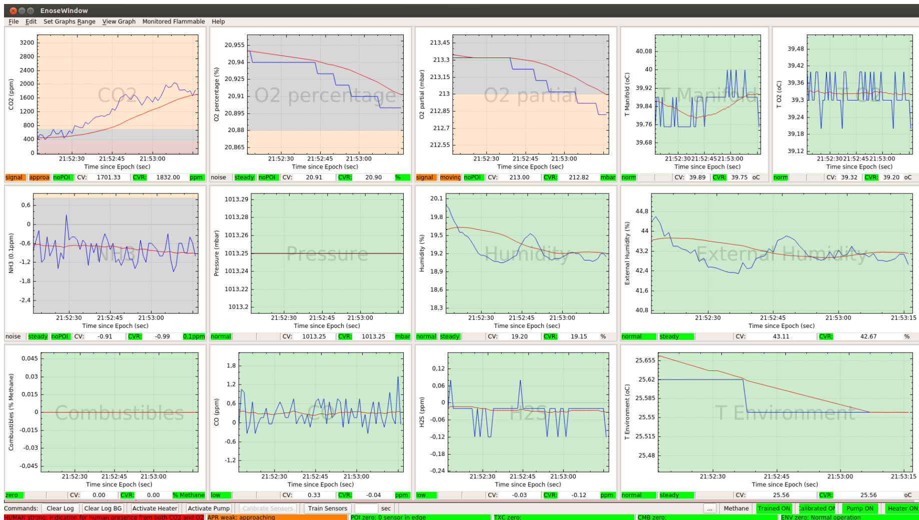
Figure 199: Human detection data with the e-nose mounted on the robotic platform. A strong human (global) indicator is triggered while the approaching (global) indicator is still weak.
