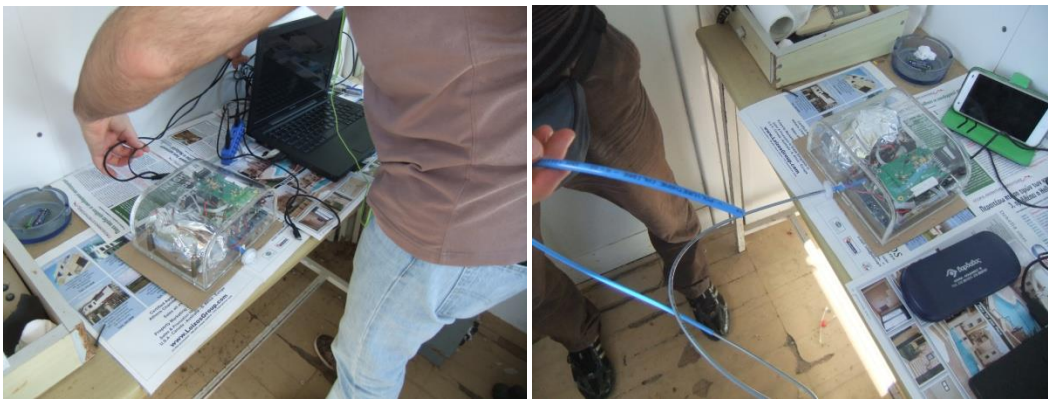
Figure 75. Left: e-nose and control interface computer. Right: e-nose and sampling tube
