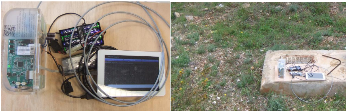
Figure 172. H 2 S detection test apparatus
