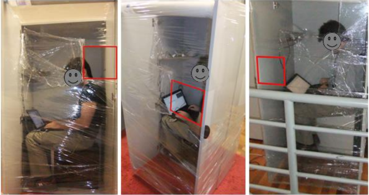
Figure 50. Various tests with different ventilation positions. Ventilation opening is 20x20cm (red shape).
