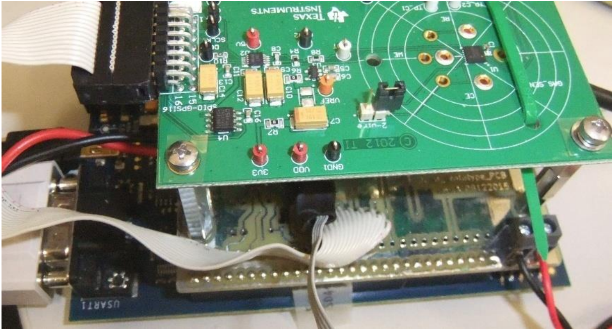
Figure 41. The assembled readout and control PCB stackup of the 2 nd prototype
