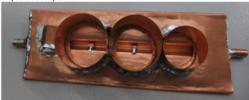
Figure 39. The lightweight and heat conductive custom manifold
