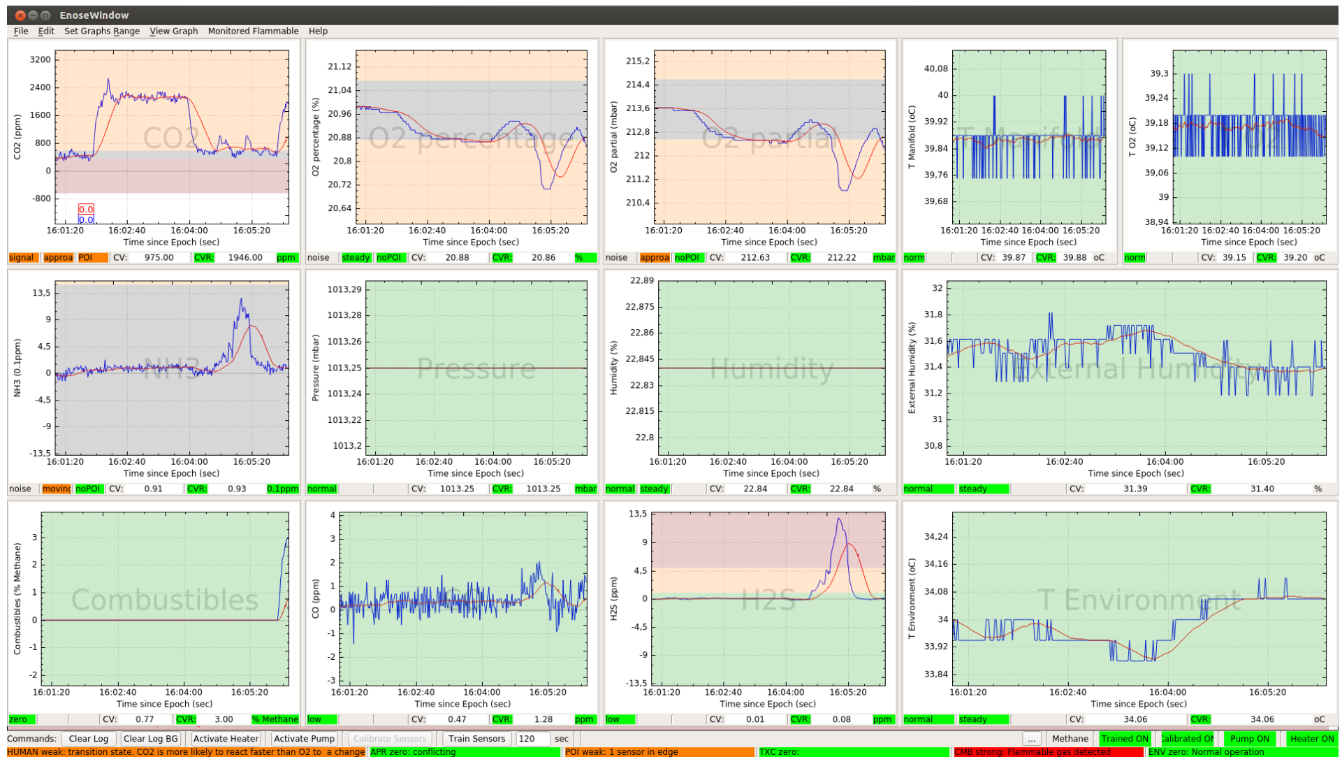
Figure 187. Case (4). Combustible atmosphere detected, with the Combustibles indicator being triggered.
