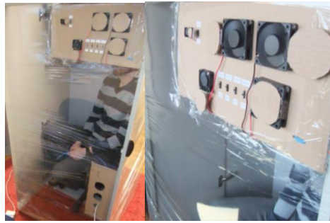
Figure 70. Left 2 fans ON~ 250lpm Right 4 fans ON ~ 1250lpm.
