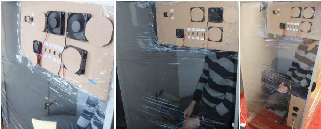
Figure 63. Left to right: 4 fans ON ~ 1250LPM. 3 fans ON ~ 750LPM. 2 fans ON~ 250LPM
