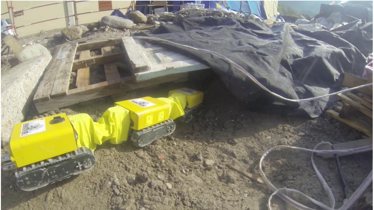
Figure 193. The search location. Entering the rubble pile, the e-nose is located on the central compartment. The air input and output interfaces can be distinguished on the side of the e-nose compartment.
