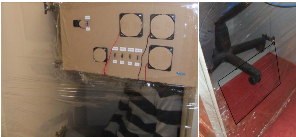
Figure 64. Left: 1 fan ON ~ 50LPM. Right: No fans ON, only 20x20cm opening.
