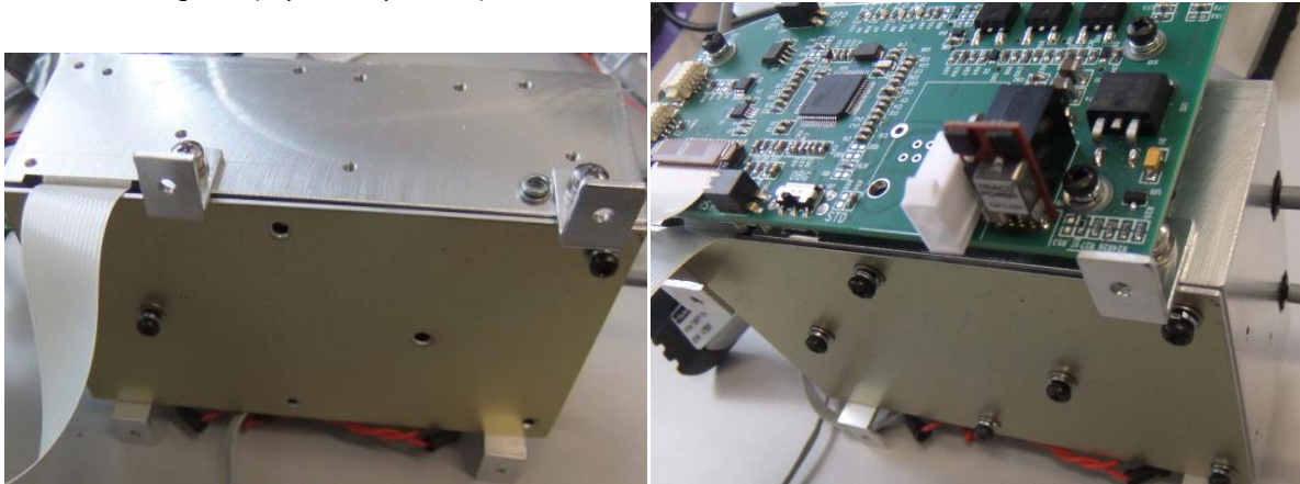
Figure 118: The assembled manifold with the control board attached to it
