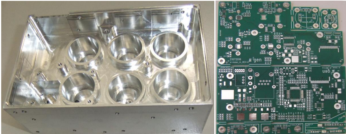
Figure 114: Bottom view of manifold with sensor inserts visible (left) and the PCB panel (right).
