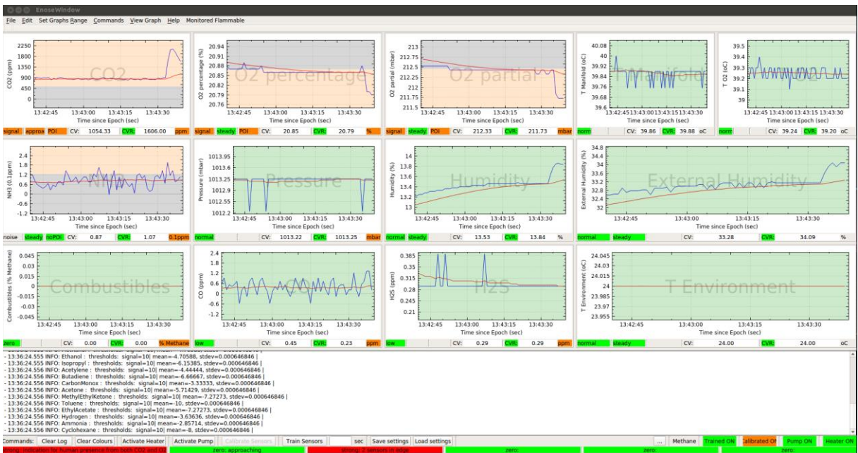
Figure 163. E-nose system output when momentarily exposed to high human presence air conditions.
