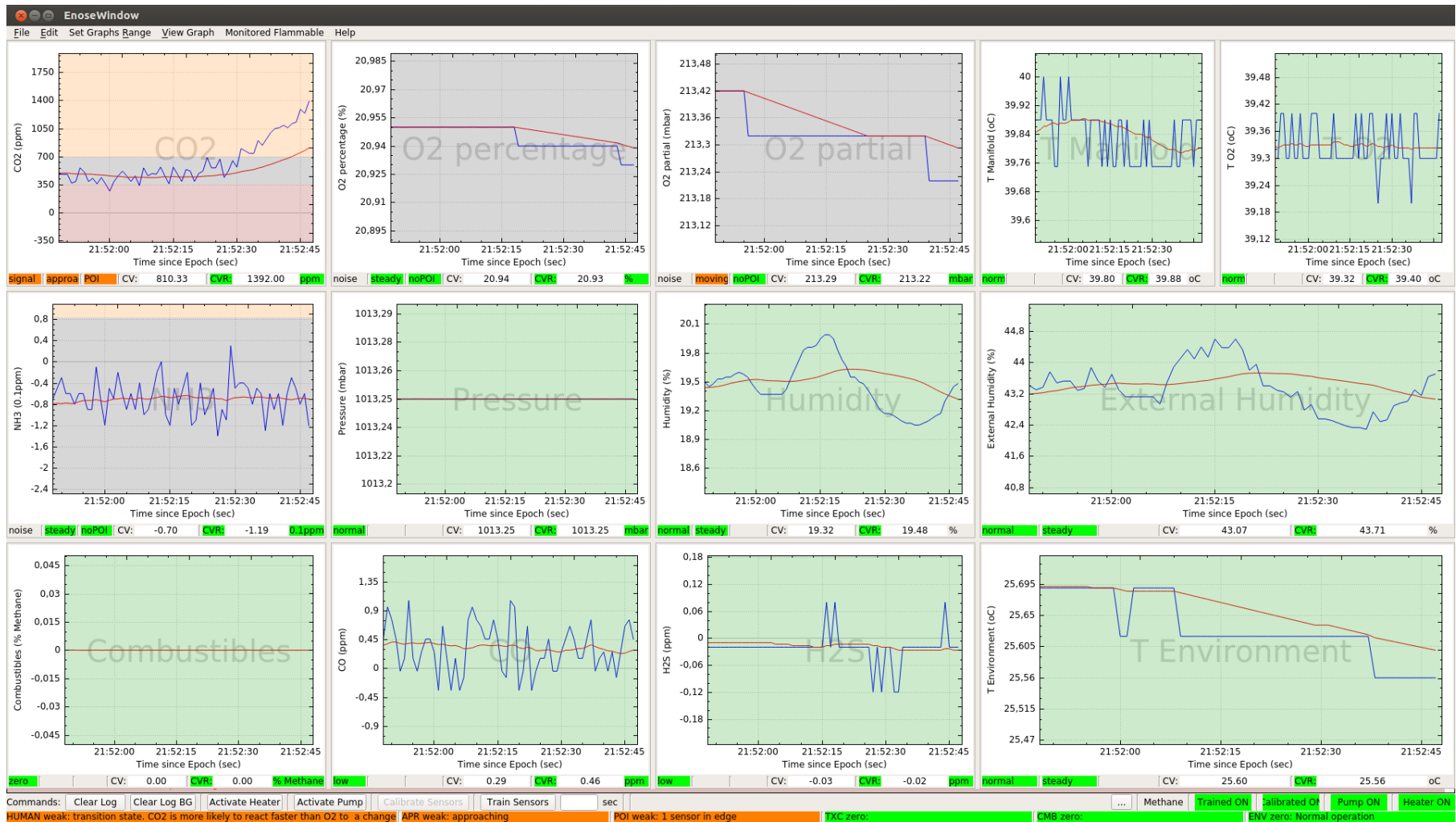
Figure 198: Human detection data with the e-nose mounted on the robotic platform. A weak Human (global) indicator is triggered, the weak Approaching (global) indicator is active, a weak Point of interest (global) indicator is triggered.
