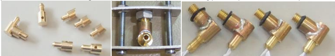
Figure 119: From left to right: machined air interface parts, custom assembly jig, assembled interfaces.
