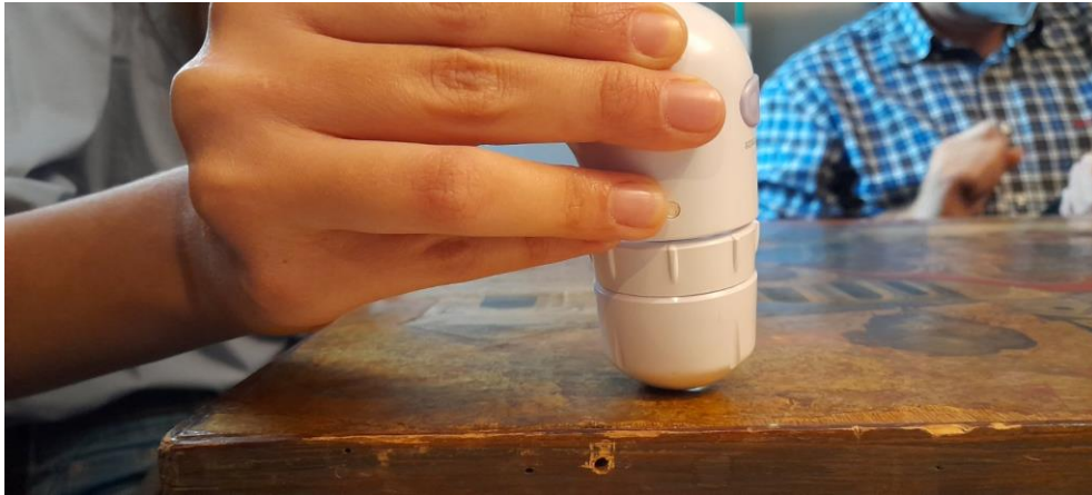
Figure 51: Image acquisition with a portable stereomicroscope (derived from personal archive Lida Kyriopoulou).
