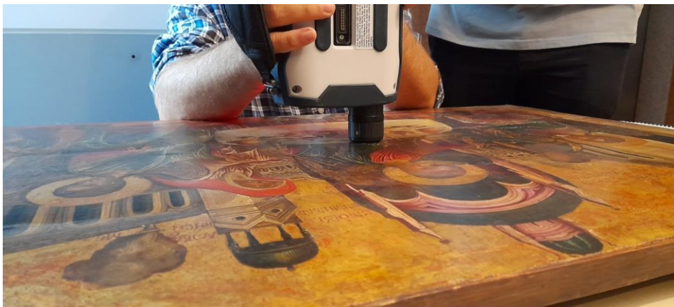
Figure 52: Analysis procedure with X-ray Fluorescence Spectrometer (derived from: personal archive Lida Kyriopoulou).
