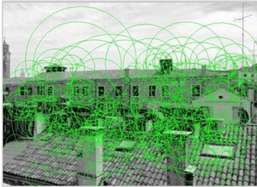
(f) Detected features using SURF in image1
