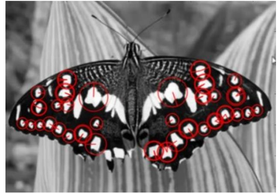
Fig. [15] SURF works like a blob detector . In the image above, it detects the white blobs on wings of the butterfly.
