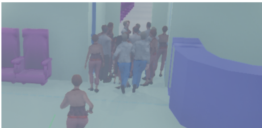
Figure 47. Congestion and Arch Formation in front of a Door (low visibility because of moderate smoke).
