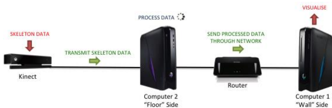
Figure 4-10. Communication process through hardware components.
