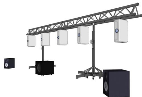
Figure 3-2. c. LIT Backstage Architecture includes five projectors and an audio system.
