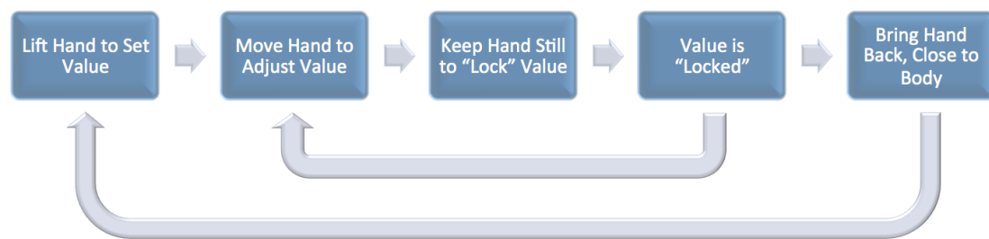
Figure 4-15. Sequence of actions a user has to perform to set a value on the HEAL interface.
