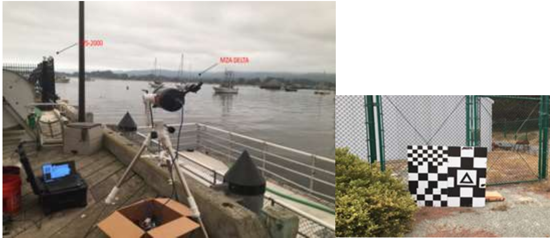
Figure 2.3 The MZA DELTA telescope and the Ambient WS-2000 weather station located on the Coast Guard Pier (left) and the target board (right) [J7].
