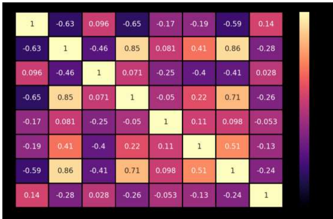
Figure 6.2. Matrix of linear correlation coefficients for measured meteorological parameters and received signal strength.
