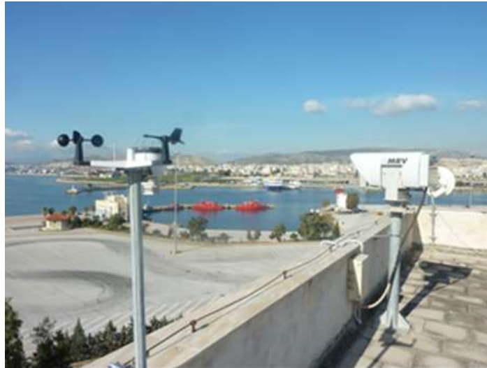
Figure 5.3. The MRV TS5000/155 FSO system on the Hellenic Naval Academy and the co-located ambient weather WS-2000, weather station [J1].
