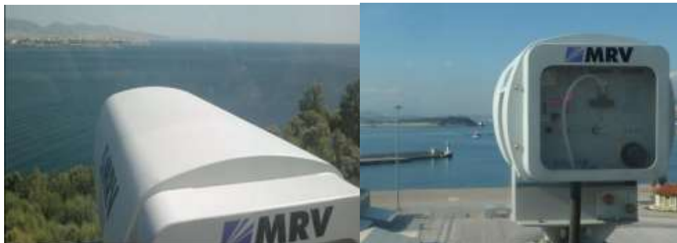
Figure 5.2. The FSO link from the Psitalia Island (left) and the HNA' building (right) point of view [J1].
