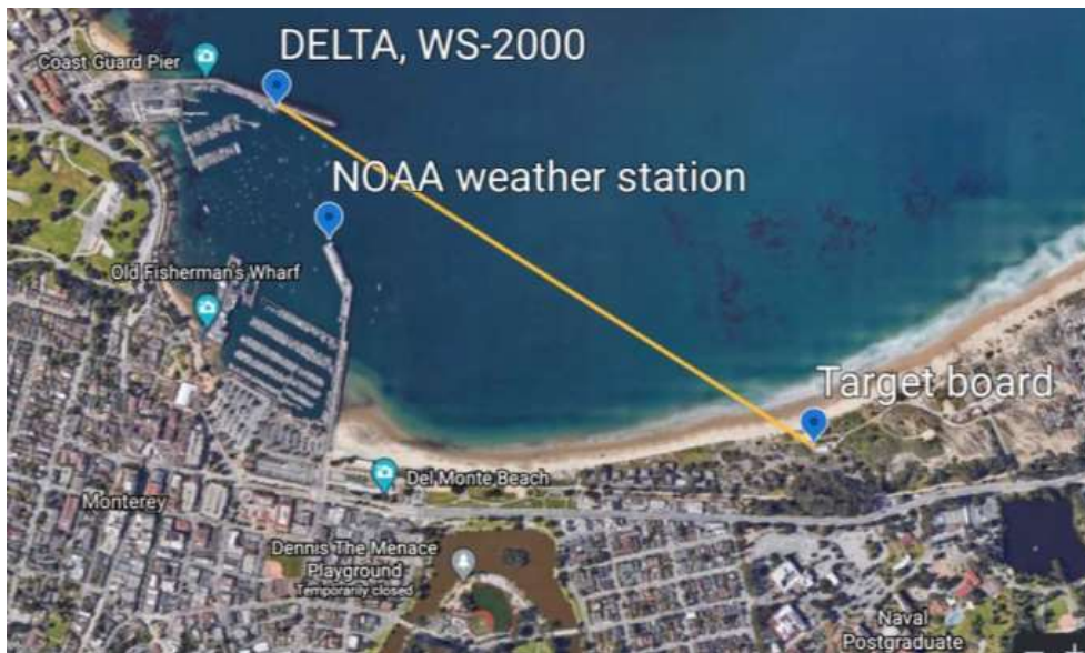
Figure 2.5. The maritime path over Monterey Bay, CA. The MZA DELTA telescope was located on the Coast Guard Pier and the target board on a coastal bluff [J7].
