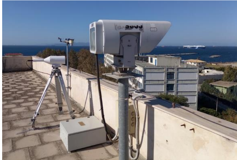
Figure 7.16. The MRV TS5000/155 FSO system, co-located with the BLS450 scintillometer and the ambient weather WS-2000, weather station on the roof of the laboratory building of the Hellenic Naval Academy.
