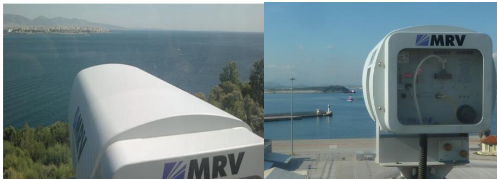
Figure 5.2. The FSO link from the Psitalia Island (left) and the HNA' building (right) point of view [J1].
