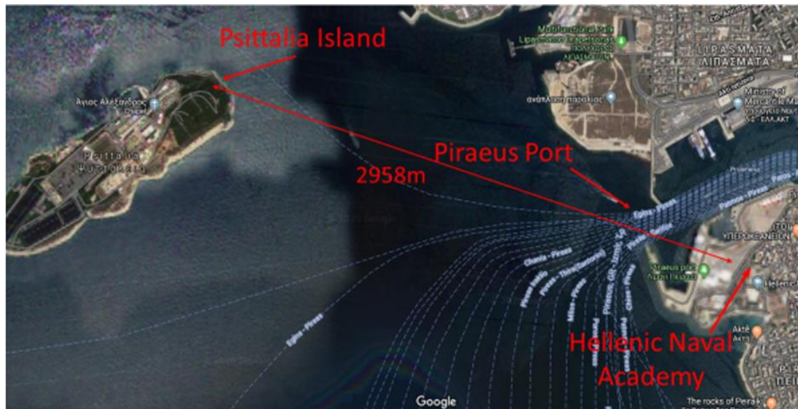
Figure 5.1. The laser communications link located across Piraeus harbor entrance [J1].
