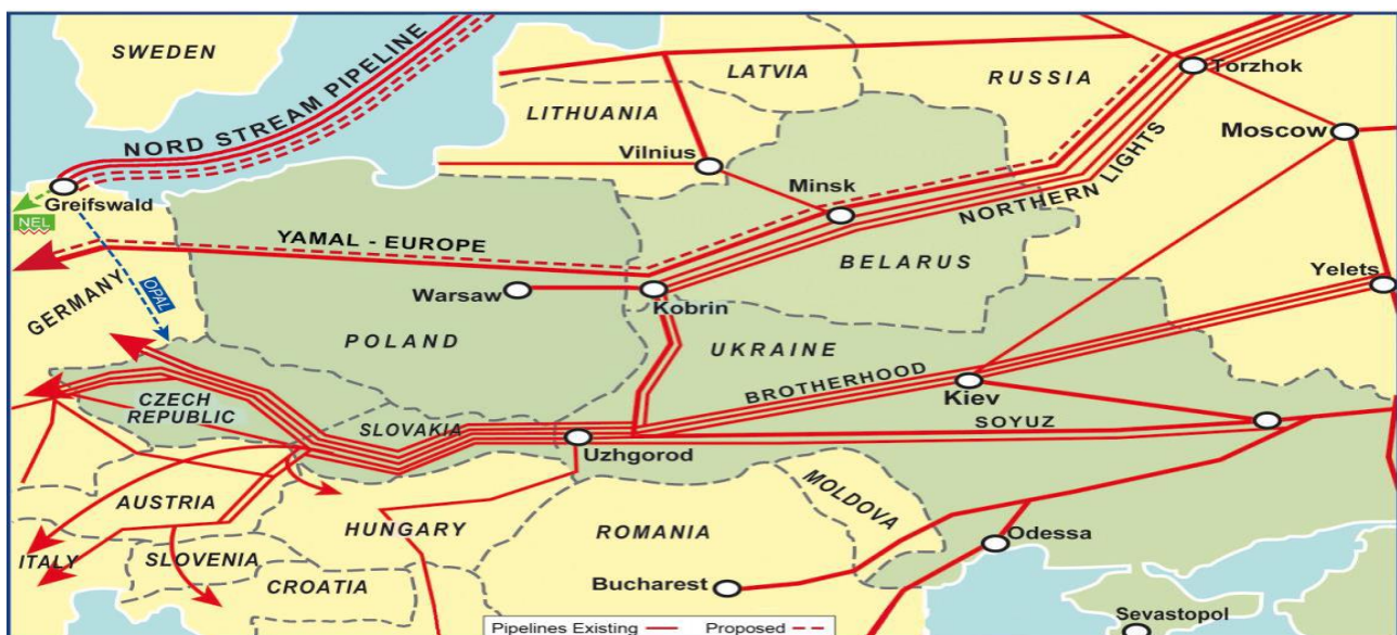
Fig.2.2 Key Russian gas export pipelines to Europe: Brotherhood and Northern Lights
