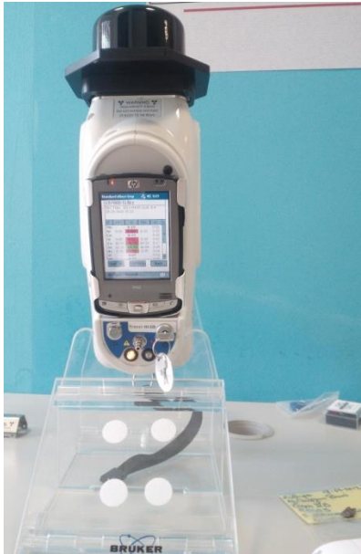
Fig.8: The portable X-ray fluorescence device (pXRF) which was employed for this study.
