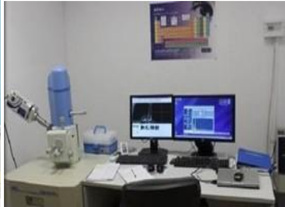
Fig.9: The SEM JEOL system coupled with an EDS by Oxford Instruments and software by INCA which was employed for the bulk compositional analysis in this study
