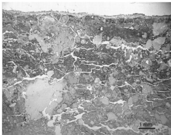
FIG. 3. Photomicrograph of a plastered floor with large quantities (30-40%) of lime inclusions and horizontal fissuring produced by compaction on the surface of the floor.
