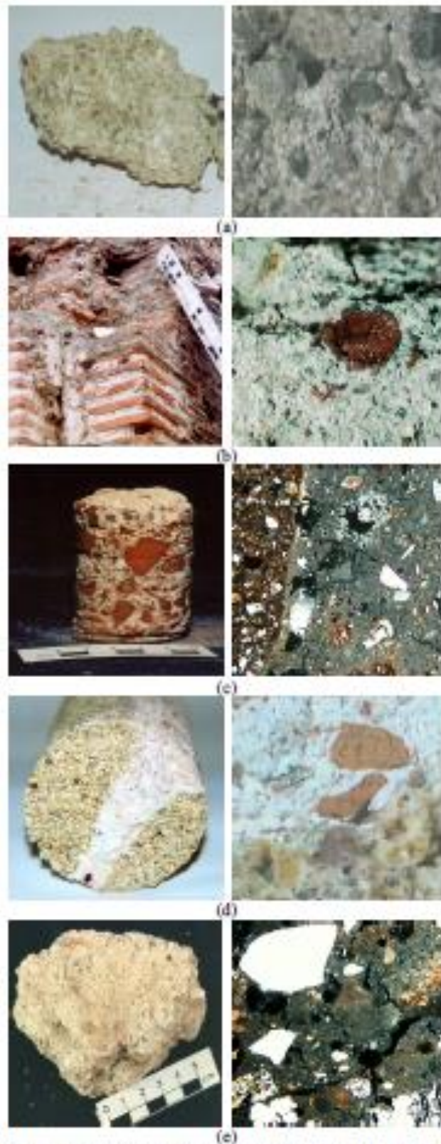
Fig. 1 Macroscopic and microscopic photos of structural mortars from various historic periods: (a) Hellenistic (Archaeological site of Lagras, 4th C BC); (b) Roman (Galerius Palace, 3rd C AD); (c) Byzantine (Saint Sophia, Thessaloniki, 8th C AD); (d) Ottoman (Bezestenli, 15th C AD); (e) Medieval (Medieval city of Rhodes, 15th C AD).
