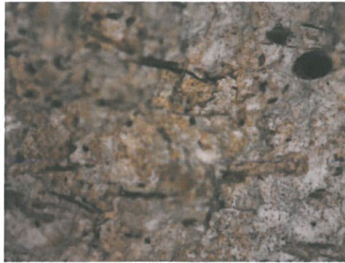
Figure 3: Sample 10, magnification x50. Plenty of pores discernible.
