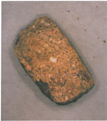
Figure 2: Sample 3, LED photo magnification x10. Homogeneous mortar with inclusions.
