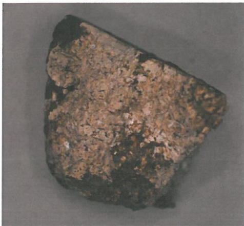
Figure 5: Sample 10, LED magnification x10. Probable fine thin layer below the pigment.
