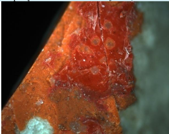
Fig.207 The upper part of the sample #9. Two layers of a red pigment (personal archive Th. Mafredas)
