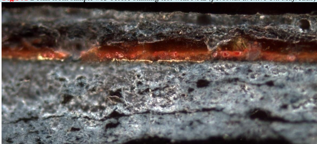
Fig.302 Detail from sample #13 after staining test with NA2 ( personal archive Th. Mafredas )
