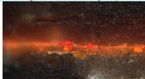
Fig.297 Detail. The pigment layer. It could be discerned the pigment grains (Magnification 50X) ( personal archive Th. Mafredas )
