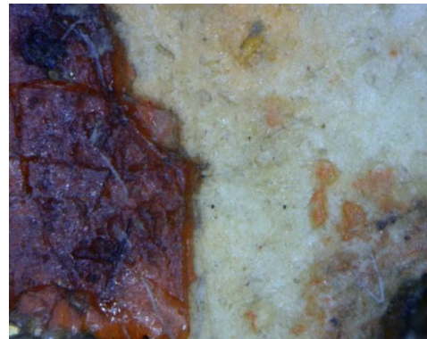
Fig.200 Thin layers of red pigment and gesso (Magnification 210X) ( personal archive Th. Mafredas )
