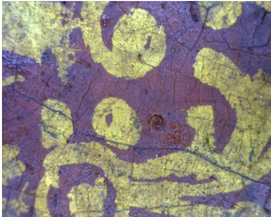
Fig.170 Detail of the decoration of the metal with red pigment over the gold layer (magnification 60x) ( personal archive Th. Mafredas )
