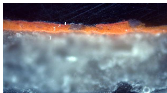
Fig.210 The stratigraphy of the sample #9. Four different layers (personal archive Th. Mafredas)
