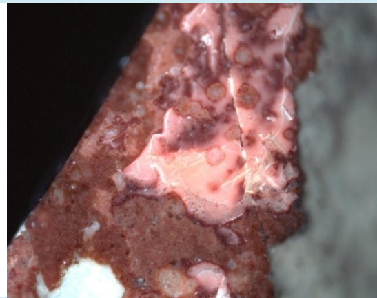
Fig.208 The upper part of the sample #9. Two layers of a red pigment under UV radiation (personal archive Th. Mafredas)
