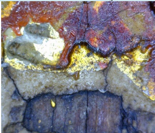
Fig.81 The thickness of the layers in DM12. Magnification 60X ( personal archive Th. Mafredas )
