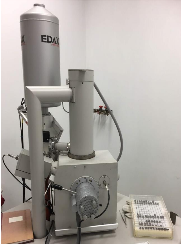
Figure 8: SEM used in this thesis research (FEI, Quanta Inspect D8334 SEM coupled with an EDS at the NCSR “Demokritos” in Athens.
