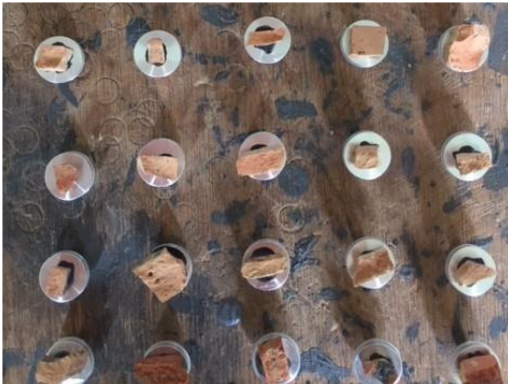
Figure 9: Samples used in this study being attached to the target holder by a conducting glue.
