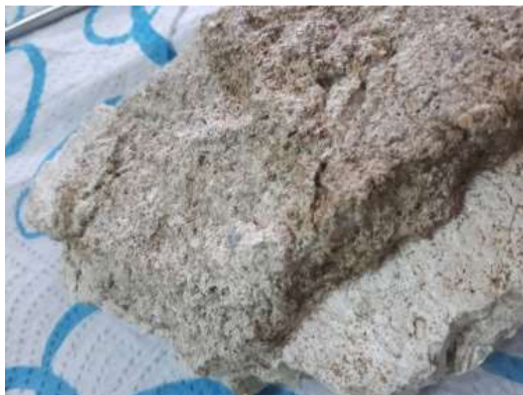
Figure 21: Underside of a wall mosaic fragment showing different layers, with the more fine white plaster seen at the bottom right side of this image. Photo taken by Paige Van Tassel.
