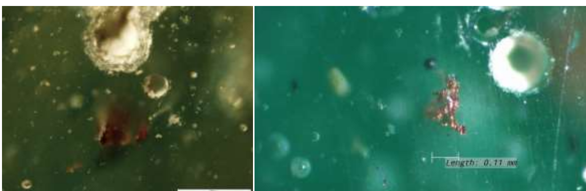
Figure 33: Blue tesserae-10 on the left and Blue tesserae-9 on the right showing copper inclusions
