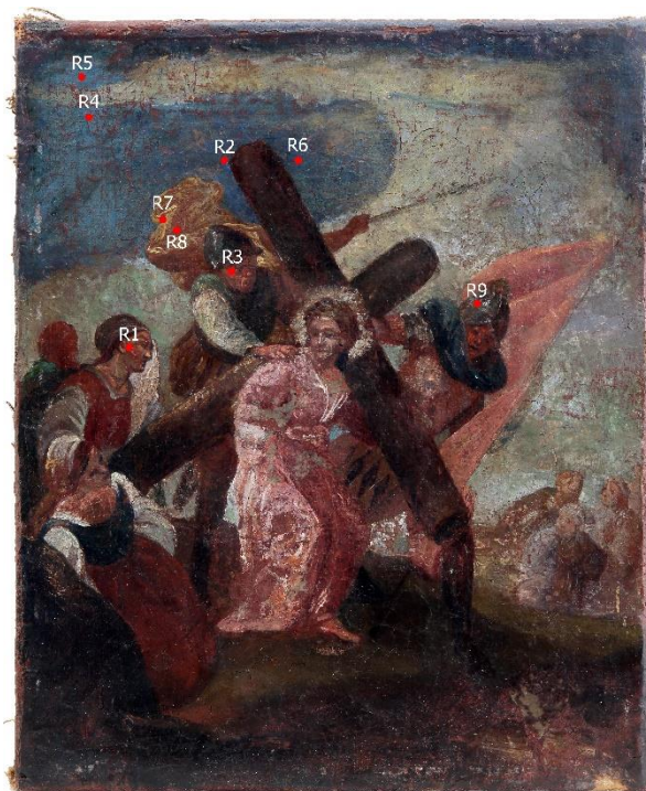
Figure 5.83 Statio VIII “Jesus and the Women of Jerusalem”. Positions of analysis by Raman spectroscopy (digital processing via Adobe Photoshop by Kesidis, Stelios).
