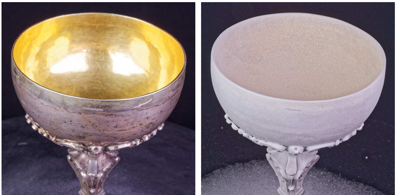
Fig. 24: Comparison of the photos of Object 1 with diffused light (left) and covered with the scanning spray (right)
