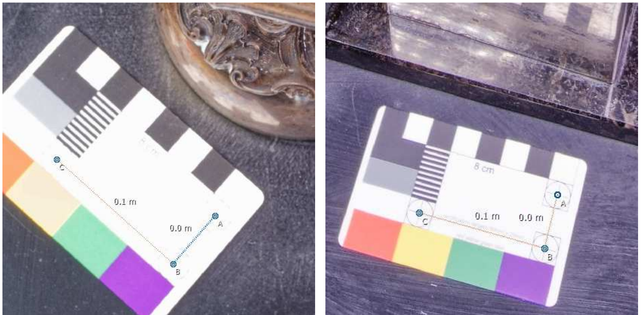
Fig. 36: Defining the distance constraints on both objects
