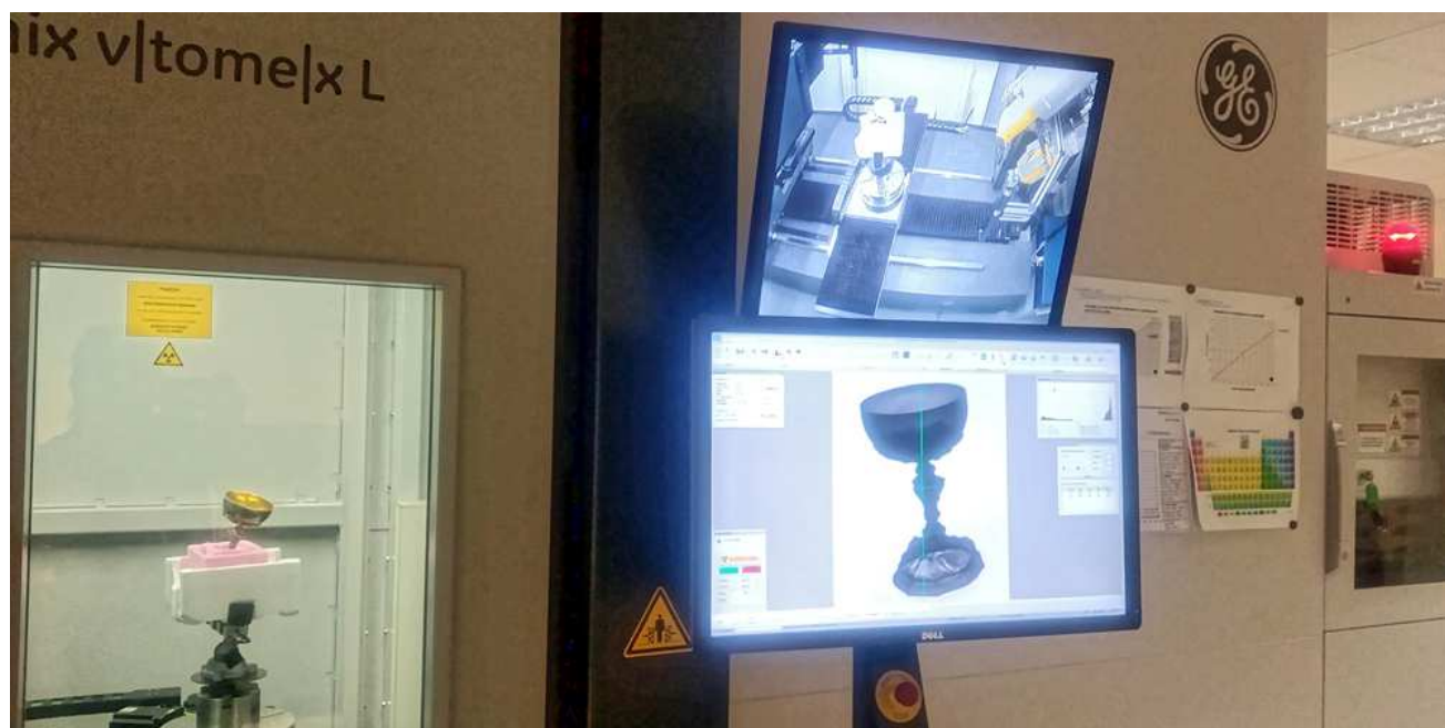
Fig. 62: Scanning of the object 1 in the micro-CT-L240
