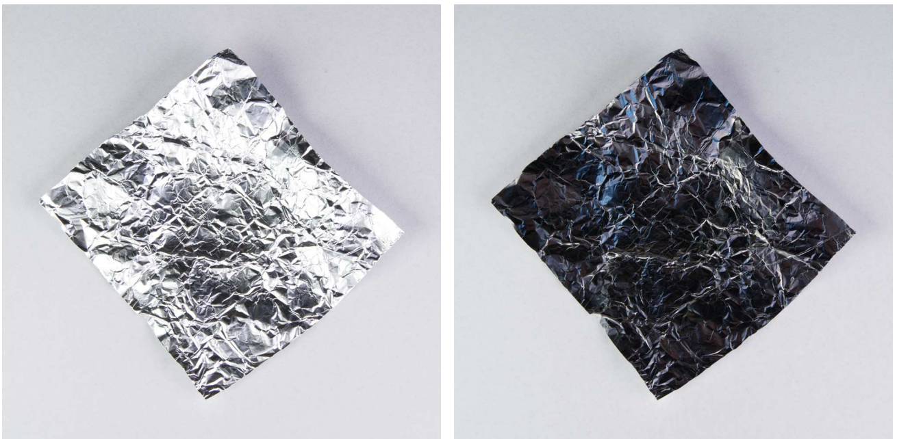
Fig. 21: Comparison of parallel and crossed filters
