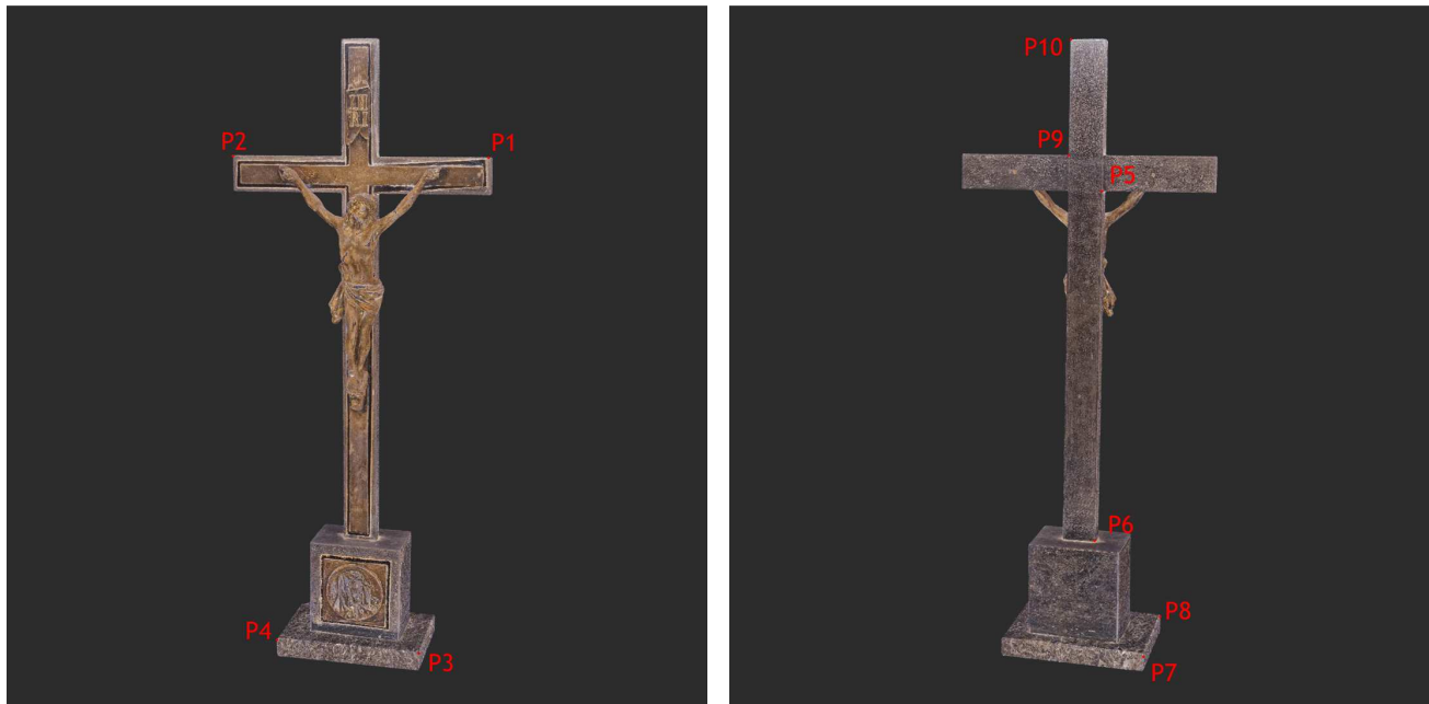
Fig. 102: Definition of measuring points on Object 2
