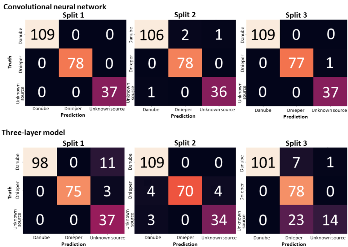
Figure 4.1: Confusion matrices for the two best performing models using three different splits at the training set. The convolution neural network (CNN) proved to be the most precise with accuracy higher than 99%.
