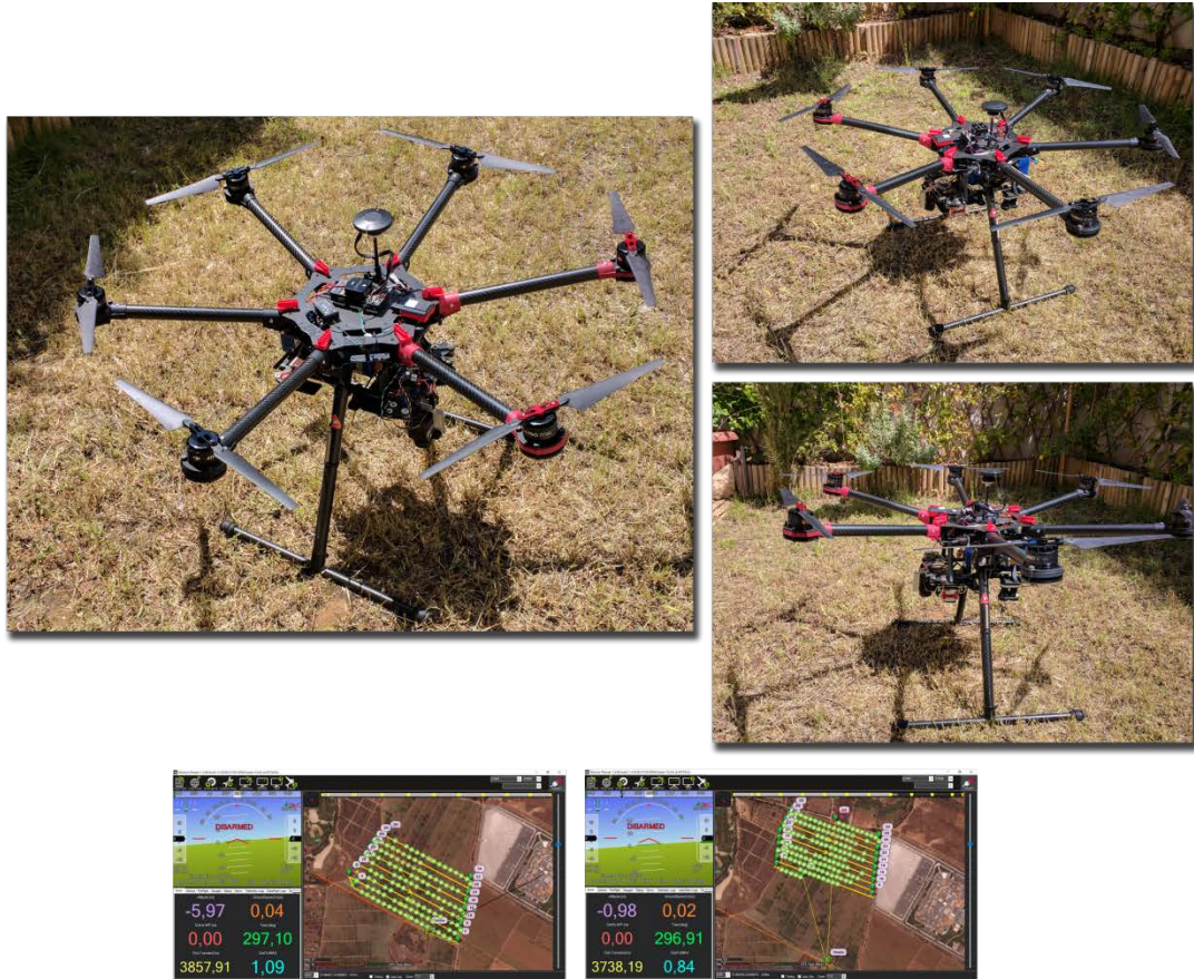
Figure 8: The UAS with payloads and 2 instances of Mission Planner after two flights
