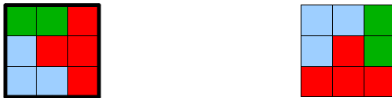
b) Recorded solution state (left), and one of the alternatives generated during puzzle initialization (recorded state rotated around the negative z axis by 90 degrees) Bold line denotes the calculated Bounding Box
