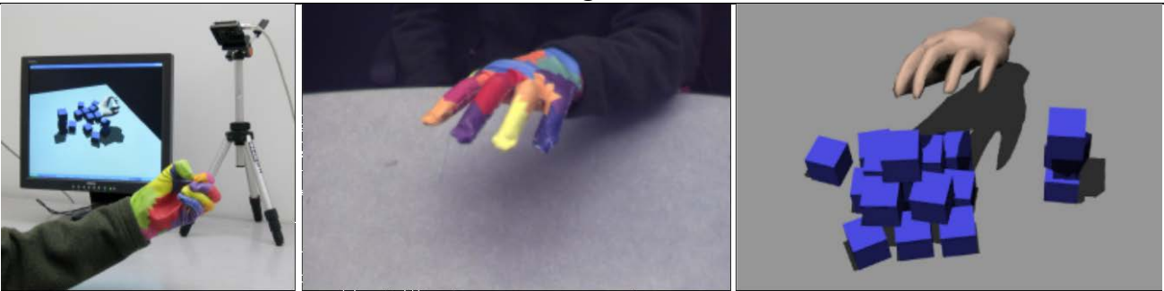
Figure 10: (Left, Middle) Color Glove tracking system, (Right) A 3D rendering of a Color Glove interaction environment
